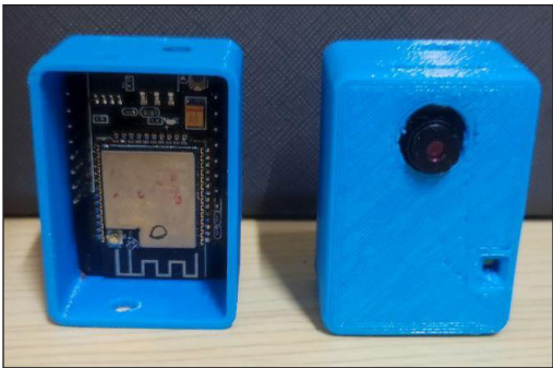
Figure 3. Front and rear view of a 3D printed casing for ESP32 CAM
